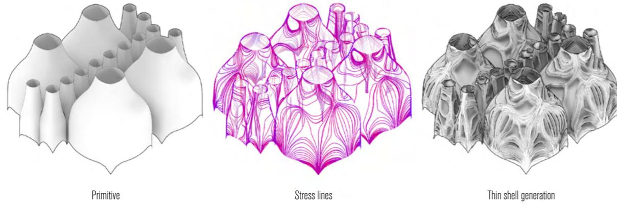
Once these spatial objects are arranged in plan, it becomes apparent that the interstitial spaces between the objects still require shelter. Thus, we generate an exterior shell system, totally self-supporting and separate from the interior shells. Both the interior shells and the exterior shells are corrugated based upon the forces against the shells under gravity. This reduces their necessary thickness, and increases their stability.
